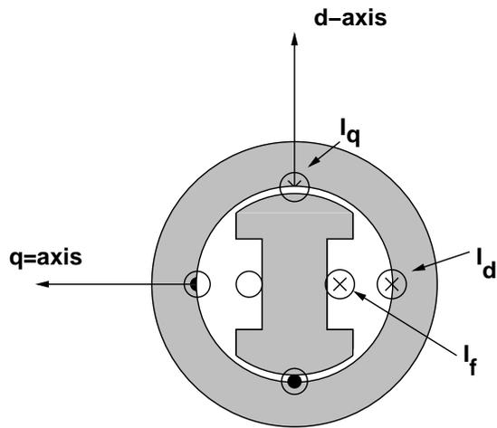
Figure 8: Cartoon of a Salient Pole Synchronous Machine
