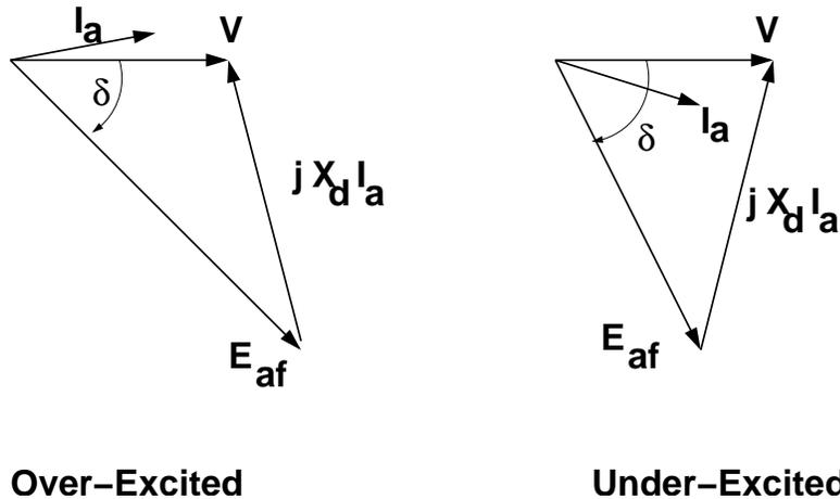
Figure 3: Motor Operation, Under- and Over- Excited
