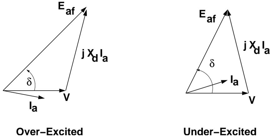
Figure 4: Generator Operation, Under- and Over- Excited
