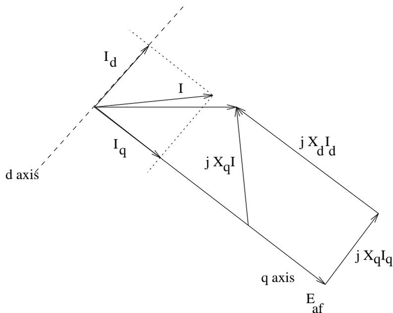
Figure 10: Phasor Diagram: Salient Pole Machine
